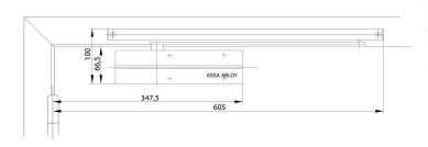
Required space on doors Left handed shown in diagram Right handed is the reverse
