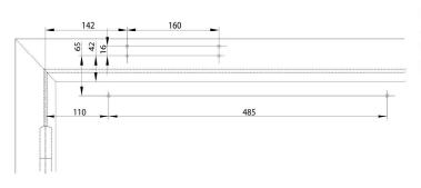
Installation dimensions with mounting plate for frame mounting on hinge side
