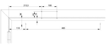
Installation dimensions for direct frame mounting on hinge side
